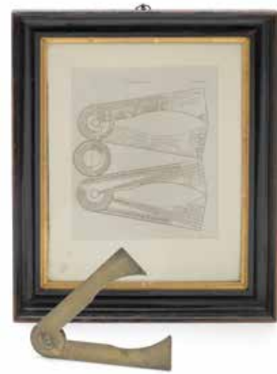
215 A WATKINS GUNNER'S BRASS CALIPER, signed Watkins, Charing Cross, London, engraved on both sides with linear and non-linear scales for the calculation of barrel-bore, shot-diameter, together with an engraved bookplate of a gunner's caliper, framed and glazed, 6 in (15cm) radius (2) £800 - 1,000 €940 - 1,200 US$1,000 - 1,300 See Bonhams.com for further footnote on this lot
