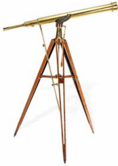
230 A 4-INCH WATSON & SONS LTD "CENTURY" REFRACTING TELESCOPE ON STAND, TP ENGLISH, CIRCA 1900, the tube with rack and pinion focusing mounted in a trunnion above brass columns with slow motion azimuth motion operated by rack and pinion and turned mahogany handle, supporting strut and folding tripod stand, in case with accessories, length of tube 53in (135cm) long £1,500 - 2,000 €1,800 - 2,400 US$1,900 - 2,500
