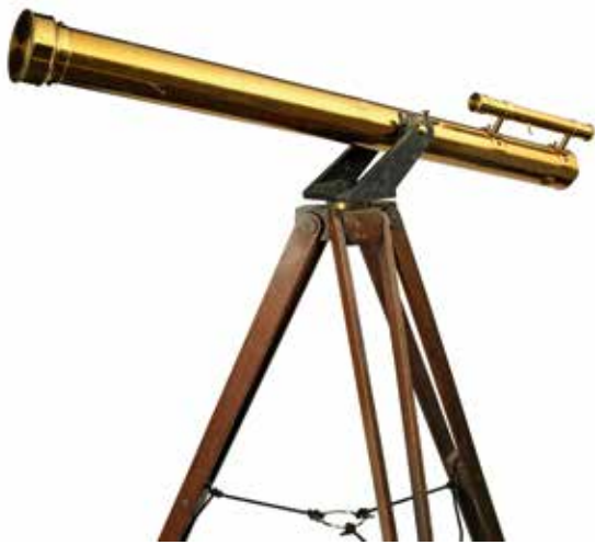
232 A DOLLOND 3-INCH BRASS REFRACTING TELESCOPE ON STAND, ENGLISH, LATE TP 19TH CENTURY, signed Dollond London 7643 , the lacquered brass tube with star finder mounted in parallel, focusing by rack and pinion, supported on a trunnion above bracket and folding oak tripod stand, in case with ocular tube and two eyepieces, length of tube 41in (104cm) £800 - 1,200 €940 - 1,400 US$1,000 - 1,500
