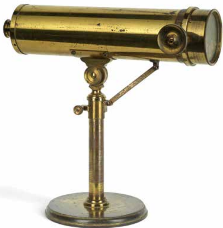
220 A CHARLES BAKER BREWSTER'S KALEIDOSCOPE, signed Brestwers Kaleidoscope, C Baker Optician 244 High Holborn, London , microcosm elements unveiling infinite combinations, the brass tube with eye-piece and objective with drum of coloured glass shards and shapes rotated by a knob at the side, supported by strut and column above circular brass base, 14 in (36cm) long x 3.5 in (8.5cm) diam, £3,500 - 5,000 €4,100 - 5,900 US$4,400 - 6,300
