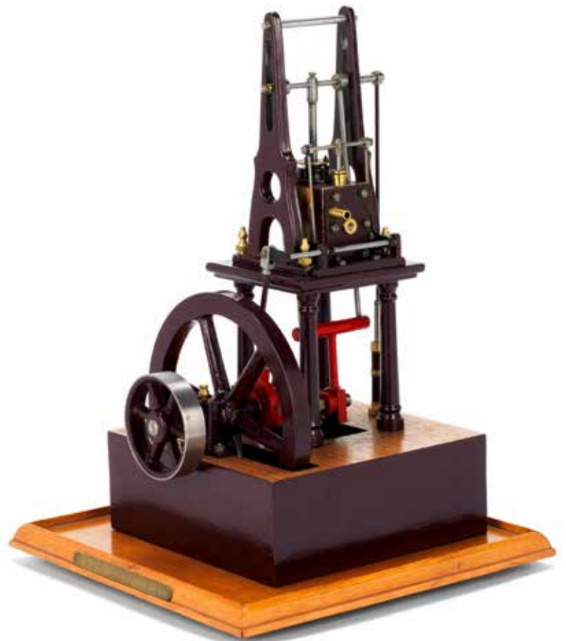
250 A MODEL OF A SINGLE CYLINDER VERTICAL STEAM ENGINE, with wooden lagged and brass bound cylinder, metal frame finished in maroon with brass finials. On wooden base, under glass case, the model 12in (30.5cm) high £600 - 800 €710 - 940 US$760 - 1,000
