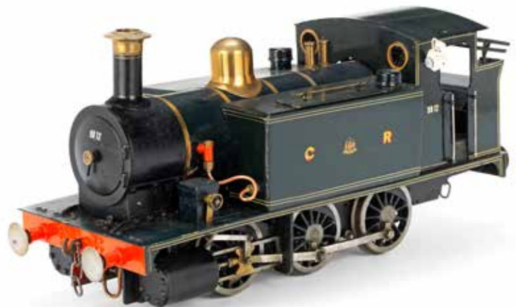
246 A WELL ENGINEERED 3 1/2 INCH LIVE STEAM MODEL OF A CALEDONIAN RAILWAY 0-6-0 SIDE TANK LOCOMOTIVE, No. 9012, with copper tubed boiler, details include hand operated gear lever, safety valves, brass dome, twin outside cylinders, drain cocks, and pipes, fluted connecting rods, hinged smoke box door, sprung buffers, finished in black livery with side lamps, brass banding and yellow lining, 21in (54cm) long £2,000 - 3,000 €2,400 - 3,500 US$2,500 - 3,800
