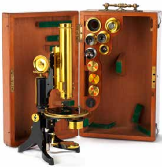
214 A J. SWIFT & SON BRASS PETROLOGICAL COMPOUND MONOCULAR MICROSCOPE ENGLISH, CIRCA 1910, complete with circular rotating stage, coarse and fine focusing and two sliding sections to the tube in fitted mahogany case with three objectives and two oculars, 13 in (33cm) high £600 - 800 €710 - 940 US$760 - 1,000
