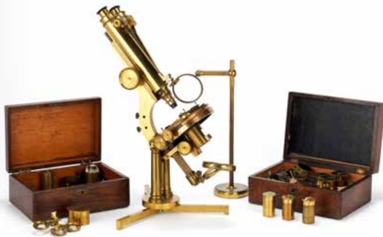
209 A SMITH & BECK COMPOUND BINOCULAR MICROSCOPE ENGLISH, CIRCA 1870, signed Smith & Beck 6 Coleman St. London No. 901 , the Lister-limb construction raised on twin columns on folding tripod base, together with accessories including bulls-eye condenser on stand, and three boxes including objectives, oculars, polariser, and relating literature and a copy of the catalogue, 19 ins (49cm) high (Qty)
